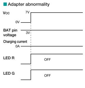
Power supply setting error (temperature detection pin open)
